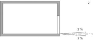
The illustrated maximum approach angles must not be exceeded. Incorrect approach angles will cause serious maneouvring & positioning problems on the parking system for which the local agency of SWISS-PARK accepts no responsibility.
